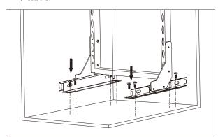
Step 6: Fix the U-iron onto the top cabinet panel with 4 tapping screws ST4. 0\*16.
